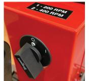
**Dual Speed**Switch between 200 and 400rpm at the flick of a switch
