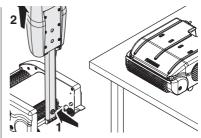
**2** Unhook the upper cover of the machine and wash it thoroughly with running water.
