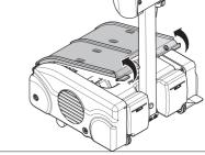
**2** Remove and empty the dirty water waste. Wash it with running water and, if necessary, use a spatula to remove any residual from the bottom.
